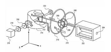
This advanced technology provides a means of NMR detection in magnetic fields near zero, thus no cryogenics required and noise associated with currents used to null the field are minimized.
