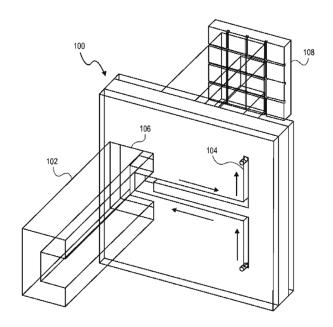
Illustrates a microfluidic device including an alkali vapor cell and a microfluidic channel where the alkali vapor cell is illuminated by a laser beam and a segmented photodiode detects the laser beam after its transmission through the alkali vapor cell according to an embodiment of the present invention. Item 100 is the microchip; item 102 is the laser; item 104 is the fluidic channel; item 106 is the alkali vapor cell; and item 108 is the segmented photodiode.
