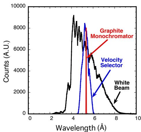
**FIGURE 1:** Time of flight (TOF) spectrum for the three wavelength resolution options. The blue curve is obtained using a NVS with rotation speed chosen to produce a mean wavelength of 5.3 Å. The black curve is the spectrum from the filtered white beam. The red curve is a calculated spectrum for the HOPG monochromator. The beam intensity is proportional to the area under the curve.
