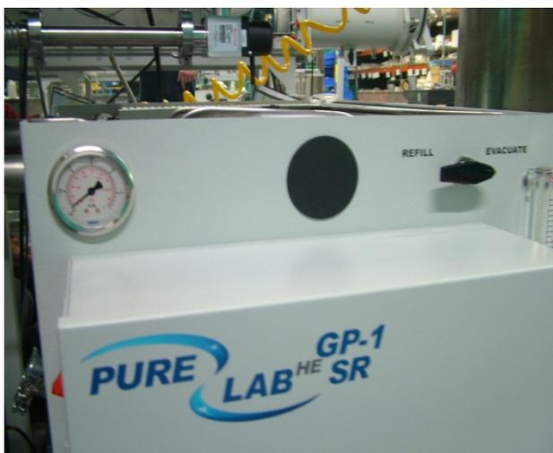
Figure 58 Evac/Refill Valve at Evacuate
