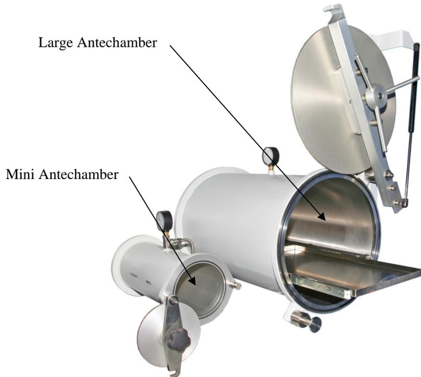
Figure 36 Inserting an object into the Antechamber
