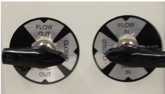
Figure 46 Oxygen analyzer valves – “Closed” position
