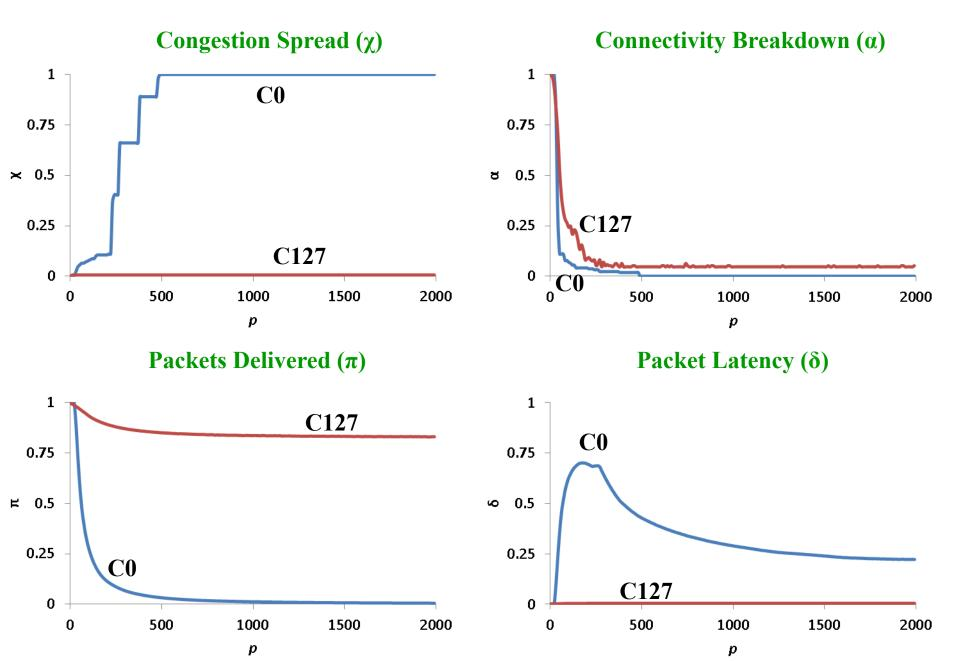
Variable speeds (VS) among router tiers, engineered to ensure adequate throughput, are *very important to model*. And modeling VS requires node classification (NC), which restricts packet injection to nodes on the network edge.
