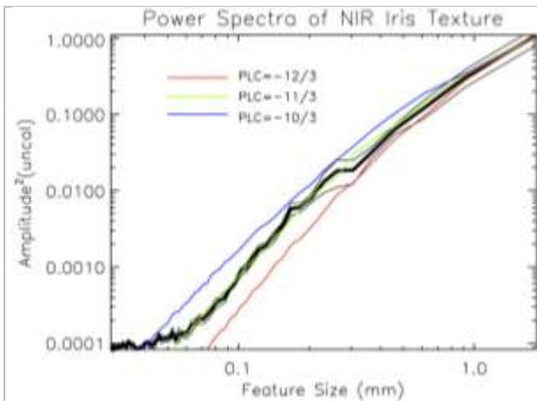
Figure 6 An example power spectra of the 2D iris texture information as recorded by near infrared imaging shows (black line) that the iris texture follows a power law distribution with a coefficient (PLC) equal to  $-11/3$ . The different color lines shows different PLC values for comparison, with the blue line showing a slightly more even distribution with PLC= $-10/3$ , and the red line a steeper distribution with PCL= $-12/3$ . (need to show the plot representative of
