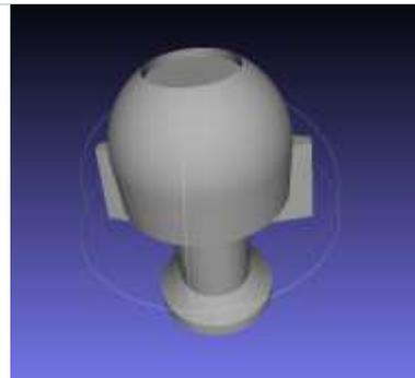
**Figure 3 An design for the eye target blank which fits inside the face mount shown in Figure 2. The piezography printed pattern and cornea simulation solutions fits inside the front facing indentation in the design. The reflective properties of the 3D printed model is similar to that of the human sclera as seen in near-infrared wavelengths.**
