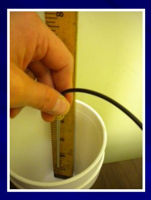
Mark the spot where the top of the probe just sticks above the rim of the cup by wrapping it with a rubber band
