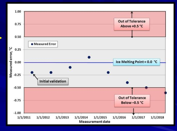
In the example control chart, we can see that a logger was validated at the ice point on an annual basis. From 2011-2017, the logger remained in tolerance, with a measured error  $\leq \pm 0.5$  °C
