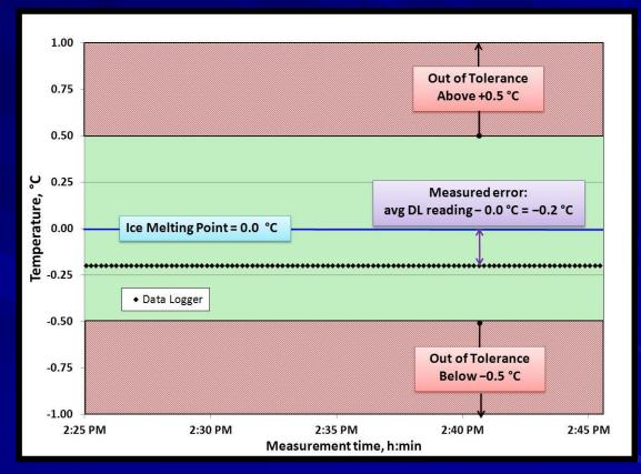
If the measured error falls within the specified accuracy (±0.5 °C), then the device is in tolerance and has been successfully validated at the ice melting point
