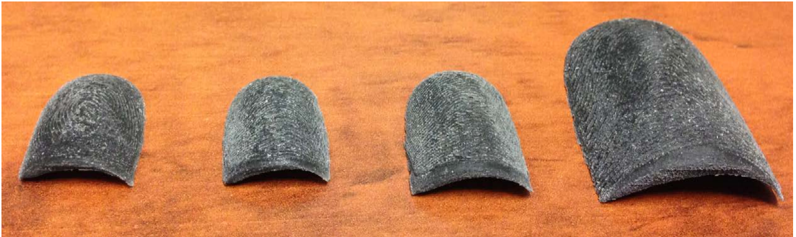
Fabricated 3D synthetic artifacts of different finger sizes and hardness
