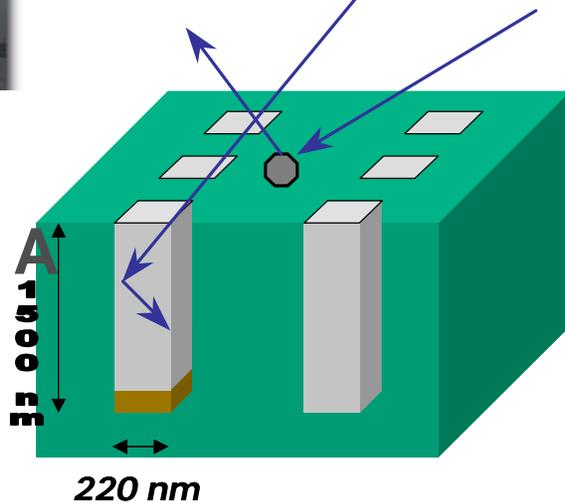
Collimated laser light (DDH) penetrates and returns from high aspect ratio structures
