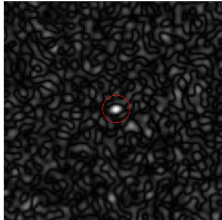
Defect easily detected in phase
