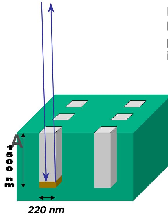
Bright field tools: Incoherent (broadband) light is poorly collimated and can only isolate surface defects well
