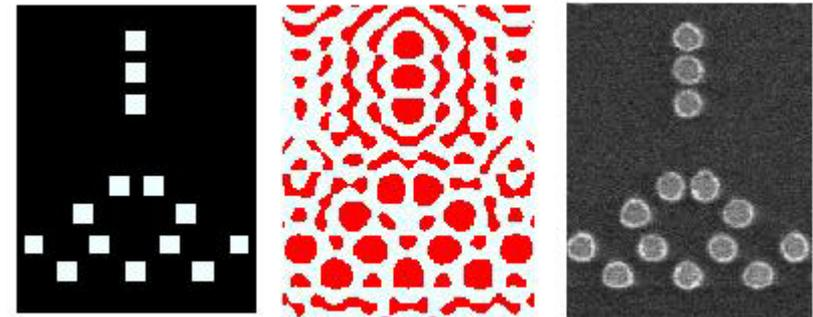
A portion of the 65nm metal 1 design (a) is converted to a pixelated phase mask design (b), where red represents  $180^\circ$  phase shift pits and green represents  $0^\circ$ , and projected by the stepper forming the resist image in (c).
