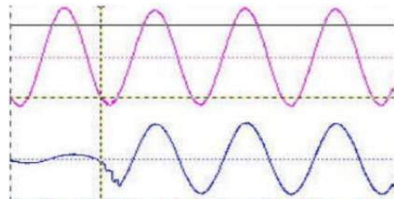
Top View: EPCC Output Voltage Sag (~5%) w/ System Motor
