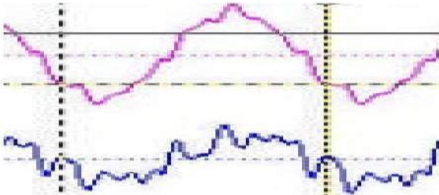
Top View: Distorted DG Output Voltage w/o EPCC Unit
