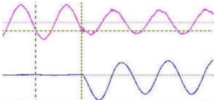
Top View: DG Output Voltage Sag (~35%) w/ System Motor
