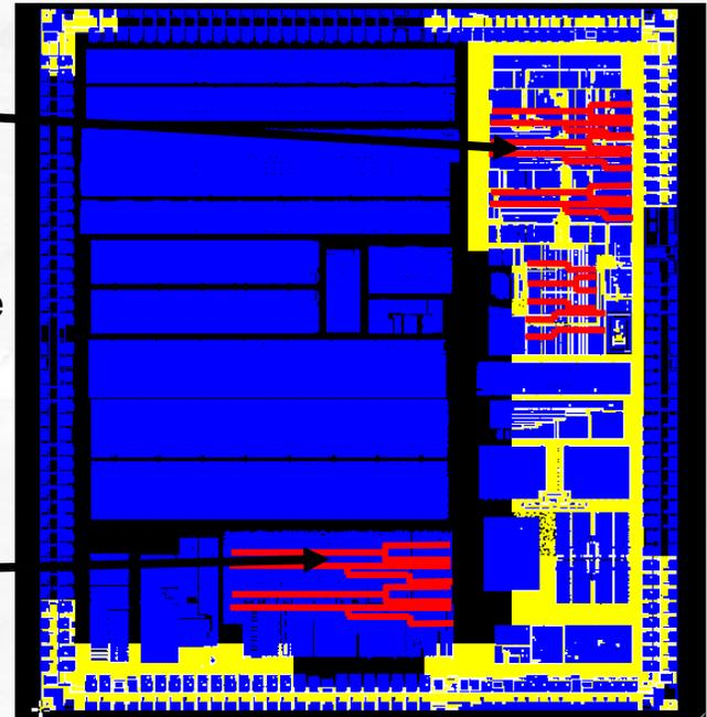
Change layout to move critical timing paths to areas without smallest errors
