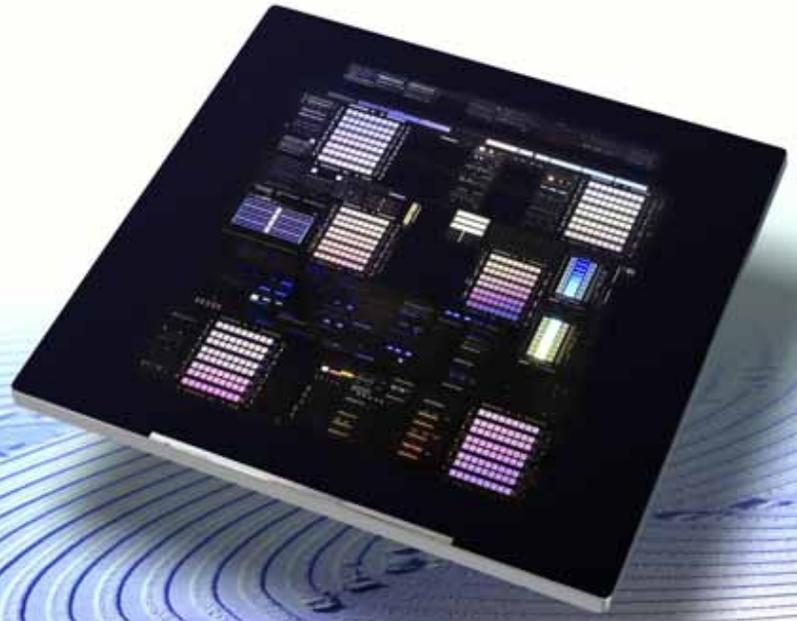
Full Field 6" EUV Mask with 100-nm node CMOS
