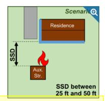
**Scenario 2** - For intermediate separation distances, directional hardening of the home facing the shed (indicated in blue) can help increase the ignition resistance of the residence.
