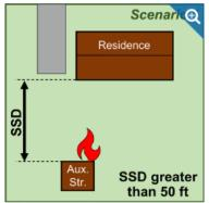
Scenario 1 - Exterior hardening of the primary residence is not necessary because the distance between the home and shed is sufficient to prevent ignition by flames. Ember protection is still needed, however.
