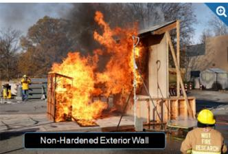
Photos from NIST experiments show the effects of a burning shed located 15 ft from the primary structure.
