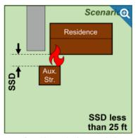
Scenario 3 - The spacing between the home and shed is too close. The fire exposure to the home will likely be too intense for exterior hardening to be cost-effective.
