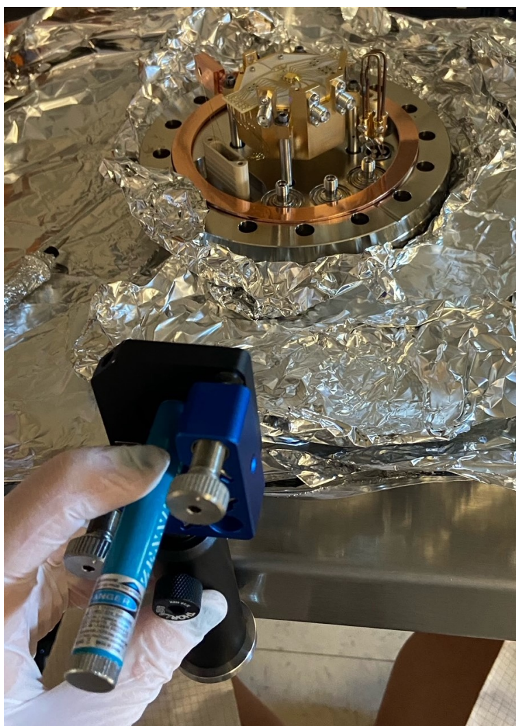
Figure A.3: The setup used to take the pictures in Fig. A.2. A 405 nm laser pointer was focused with a 150 mm lens and manually scanned over the trap surface. For the systematic evaluation of trap chips performed for the new trap candidates, the laser pointer was mounted to a stage for repeatability, and a clamp was used to hold the laser pointer button in the ‘on’ position.
