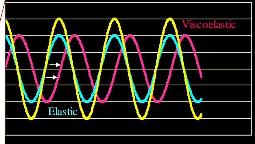
Lock In Amplifier continuously measures phase and amplitude of displacement signal and outputs to imaging system.
