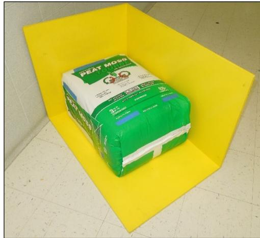
**Figure 3-1. Dimensional Measuring Frame.**
