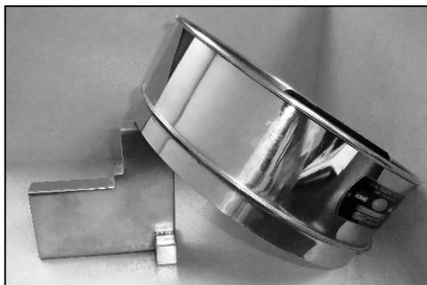
**Figure 2-3. Sieve with Tilt Block Set at 30 Degrees.**
