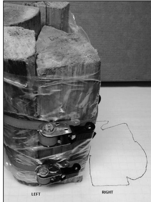
**Figures 3-15. Tracing the Perimeter of the Wood.**
