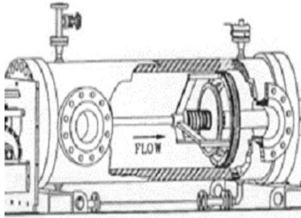
**Precision Bore Chamber & Displacer**
