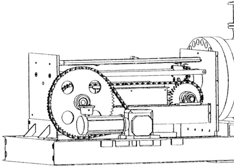
**SVP with Chain Mechanism Operation**
