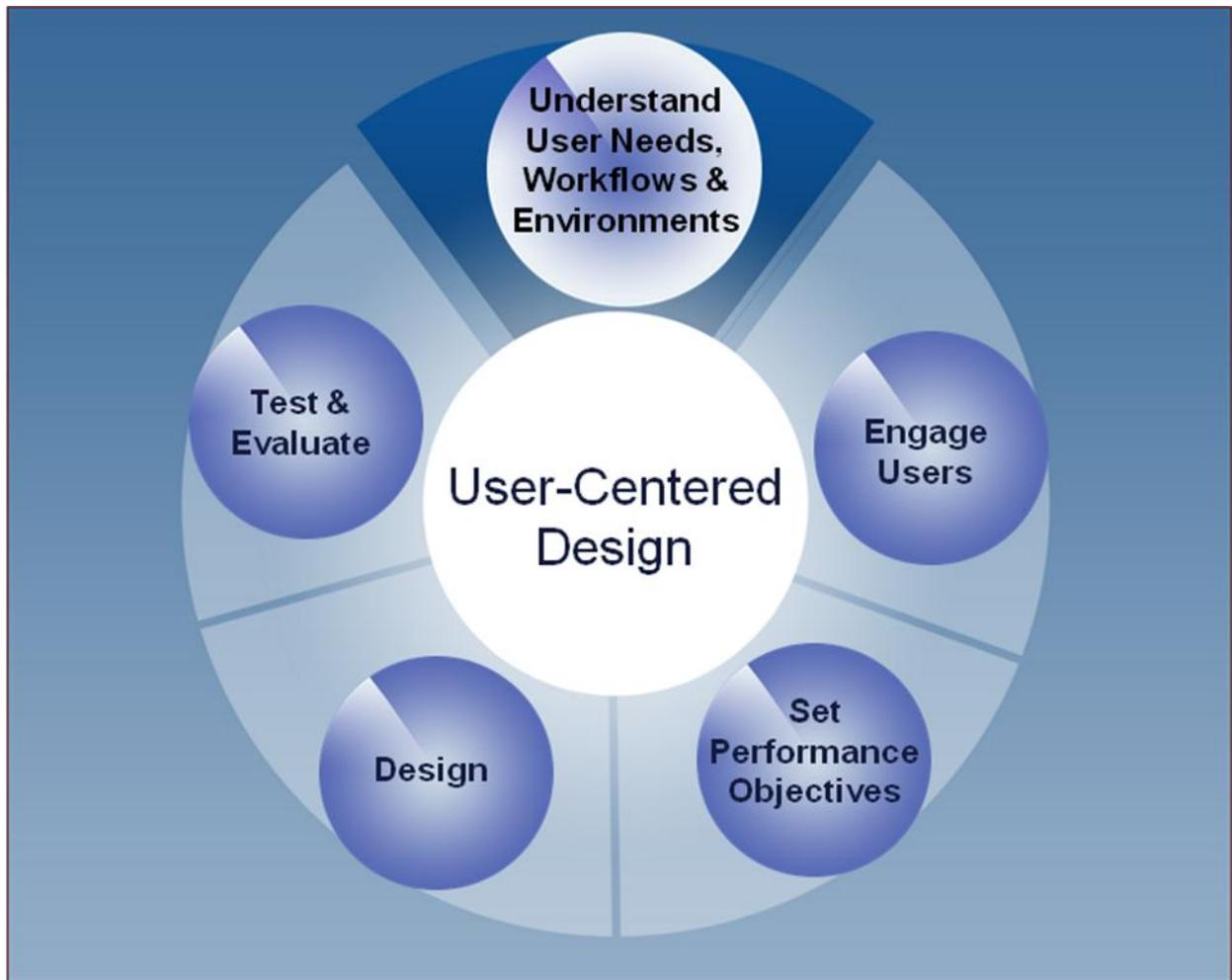
**Figure 1. UCD Process involves understanding the background of the users and the work environment, getting the users involved early in the design, setting objectives for the application, doing detailed design, testing, evaluating, and changing. The process cycles can go through many iterations at each step and can cycle repeatedly from understanding through testing.**
