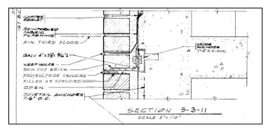
Figure 2: Third Floor Section – VWWSH Dwg 5-3, Detail 17. 1962
