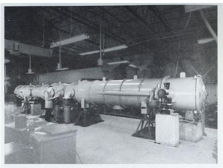
One of the new 35-foot grating spectrographs, specially built to NBS specifications, which will be installed in the new NBS Physics Laboratory. It is here shown as test-assembled by the manufacturer.
