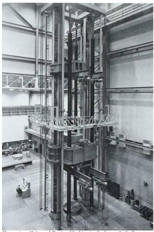
Figure A15: Universal Testing Machine in the Large-Scale Structures Testing Facility. (Source: Facilities of the National Bureau of Standards
