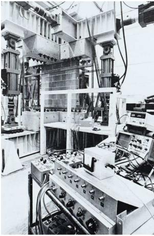
Figure A18: Tri-Directional Test Facility. (Source: Facilities of the National Bureau of Standards Brochure)
