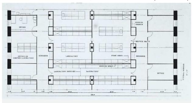
Figure A19: Schematic of laboratory arrangement. (Source: NIST)
