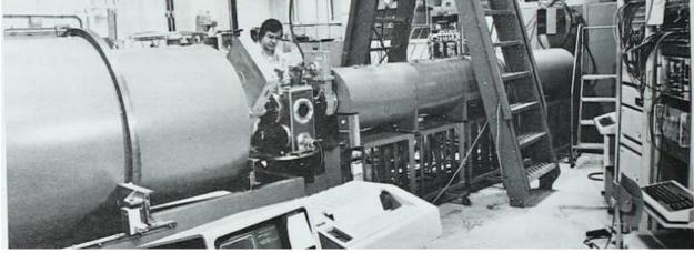
Figure A24: Small-Angle Neutron Scattering Facility. (Source: Facilities of the National Bureau of Standards Brochure)
