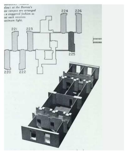
Figure A21: Rendering of a section of one of the GPL buildings illustrating the purposefully staggered doorways and windows which control natural light exposure. (Source: NIST)
