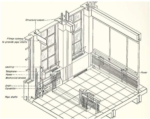
Figure A8: Diagram of laboratory modules. Piers at intervals are incorporated into the outside walls as a source of all services. Modules allow access to mechanical and electrical services while providing both natural and artificial light. (Source: National Research Council, Report on Design, Construction and Equipment of Laboratories, 1951)
