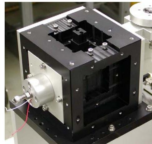
**Modularized laser interferometer**
