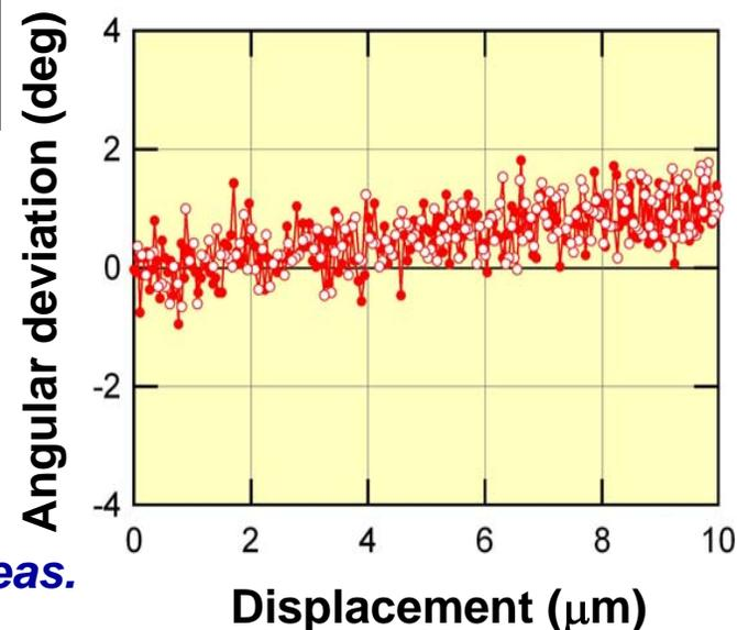
**Estimated measurement error for 100 nm :**
