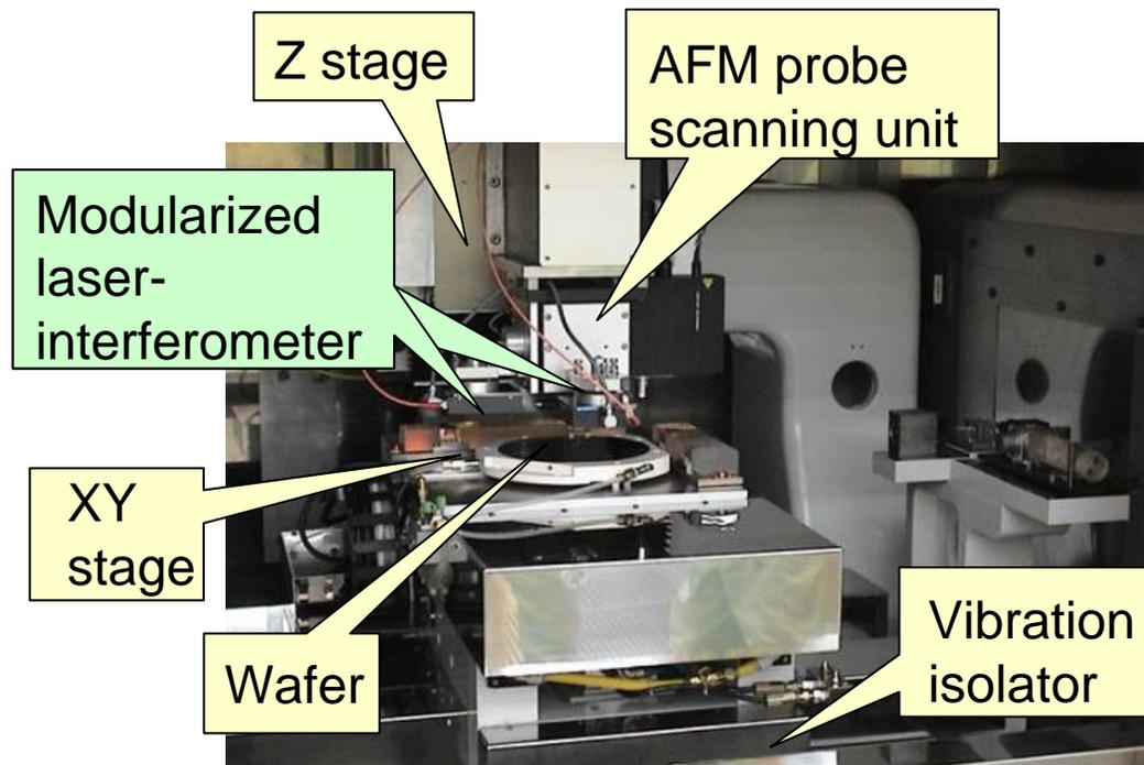
AFM probe scanner and mirror
