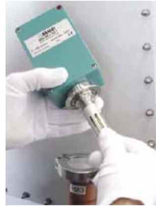
Remove KF40 clamp and blank cap.
