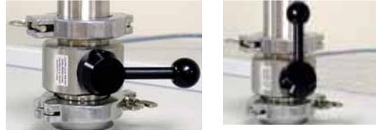
The VG valve will open and close to allow working gas to flow into the box. Once the pressure inside the box drops to a level between 1.0mbar and 8.0mbar, the valve will stay open\* providing a constant flow of gas into and out of the box.
