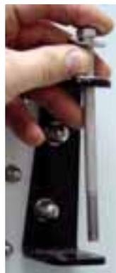
Place the hinge side of the touch panel enclosure between the openings of the bracket.
