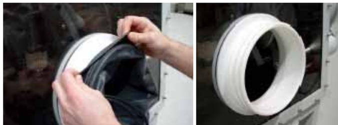
Slide the glove onto hand and insert arm into the box through the gloveport angling the thumb to a comfortable working position.
