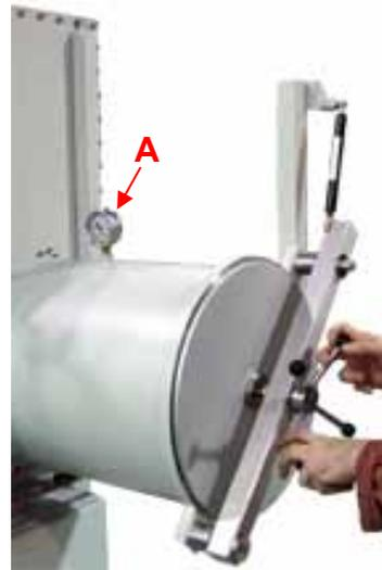
Carefully open the antechamber door by lifting it in an upward direction.
