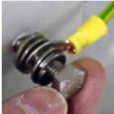
Screw the bolt back into the leg by turning in a clockwise motion.
