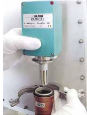
Place a blank KF40 cap over the pipe and secure in place with the clamp.
