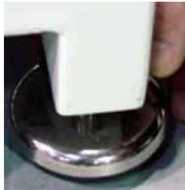
Using a 13mm wrench continue to lower the leveling feet until the casters are raised off the ground.
