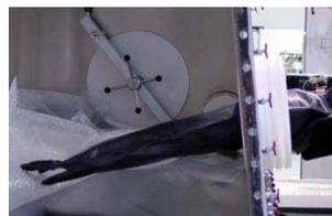
Slide hand out of the glove and work the cuff of the glove into the groove in the gloveport closest to the glass. At this time the thumb position can still be adjusted by rotating the cuff of the glove.
