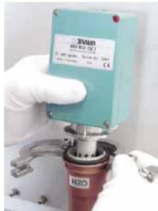
Secure in place with the KF40 clamp.
