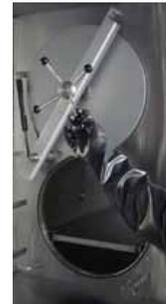
Very slowly turn the outer antechamber door handle in a counterclockwise motion until the glovebox pressure drops to a level between 1.0mbar and 8.0mbar and the VG valve stays open\* providing a constant flow of gas into and out of the box.
