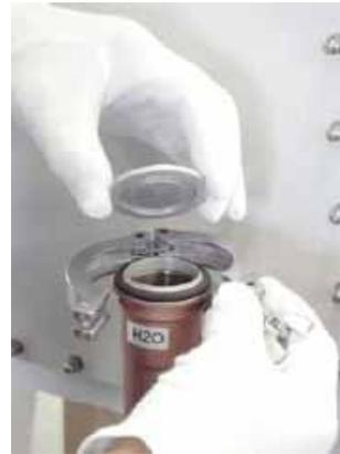
Carefully place the sensor end of the analyzer into the port on the circulation piping.
