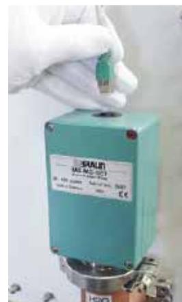
Remove clamp and analyzer.
