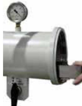
Place the materials to be used on the tray and slide the tray back into the antechamber. Replace the cover and lock into place by turning in a clockwise motion.
