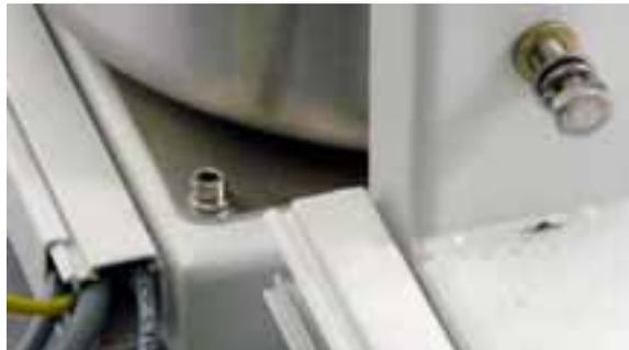
Remove the two bottom washers from the bolt.
