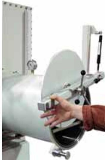
Place four fingers, two each on opposite spindles, on the door handle and gently turn in a clockwise motion until the door touches the chamber.
