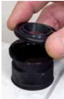
Place the oil mist filter onto the port.
