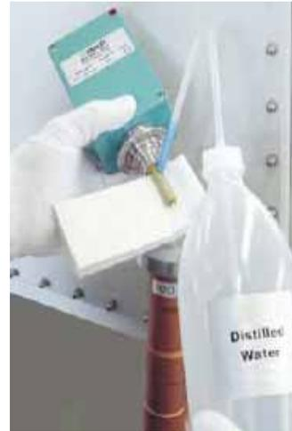
Wrap the moistened cloth around the probe. Gently and slowly spin the cloth around the probe to clean it.
