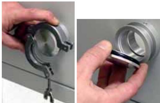
Place the o-ring on the female connector side of the feedthrough.
