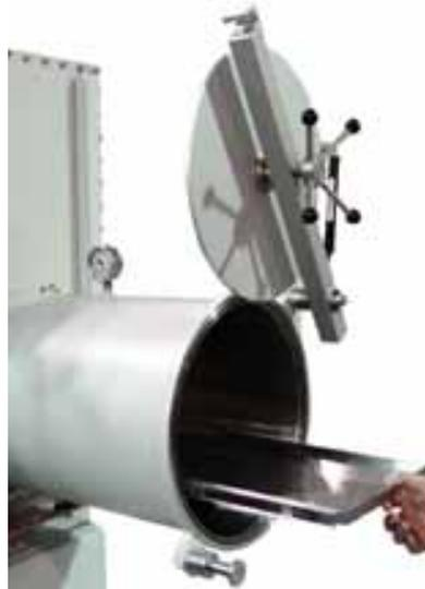
Place the materials to be used on the tray and slide the tray back into the antechamber.
