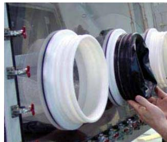
Secure the glove with two o-rings.
