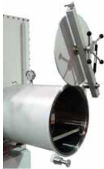
Close the outer door by pulling it down until groove at the end of the arm rests on the spindle.
