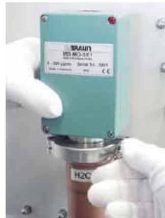
Insert the analyzer cable plug into the hole on the analyzer by pushing the plug into the hole gently until it snaps into place.
