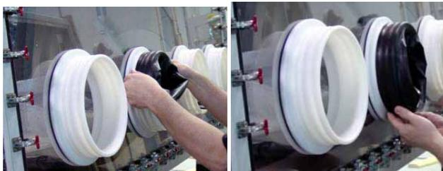
Secure the glove with two o-rings.
