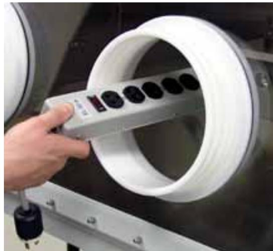
Plug the power strip into the feedthrough.
