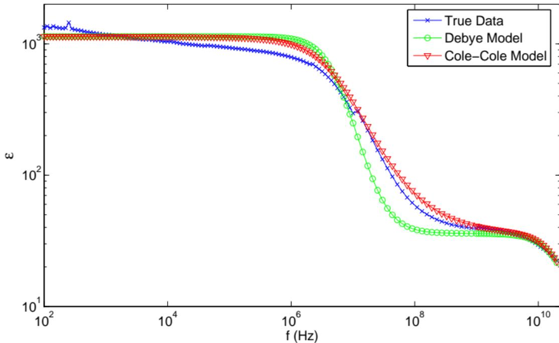
**Figure :** Real part of  $\epsilon(\omega)$ ,  $\epsilon$ , or the permittivity [GLG96]. Note: up to 10% spread in measurements was observed, but only averages were published.
