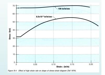
Aircraft impact lead to strain rates estimated at 100 to 1000 per second
