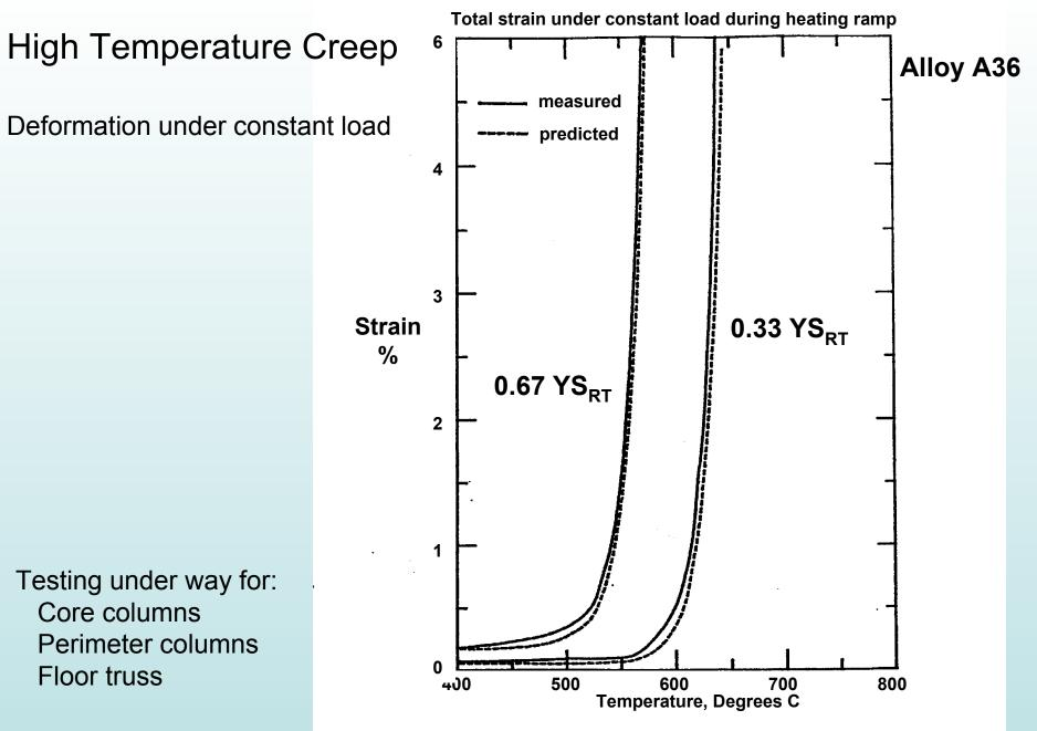
Figure 11. Measured and predicted strains during a non-linear heating rate for stresses of 1/3 and 2/3 of the room temperature yield strength.
