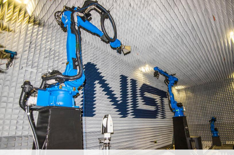
The NIST Antenna Metrology Project performs measurements on advanced antenna systems operating in complex environments. For example, the Large Antenna Positioning System (pictured) is supporting the development of next-generation 5G wireless and spectrum sharing systems.
