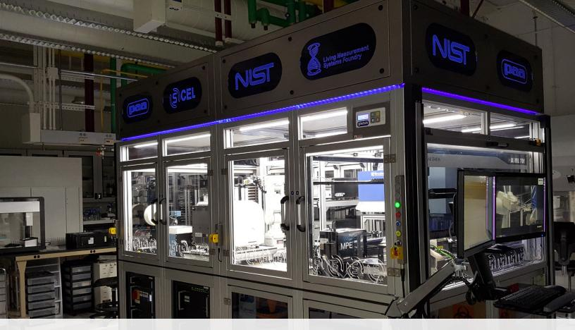
The NIST Foundry for Living Measurement Systems is a fully integrated, high-throughput system to automate common tasks in synthetic biology research from liquid handling and multi-well plate measurements to flow cytometry and nucleic acid sequencing. Credit: NIST
