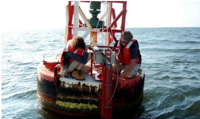
Max Ivanov and Scott Mowery with NOAA's Center for Operational Oceanographic Products and Services install an improved current sensor system on a navigation buoy in Chesapeake Bay. The system transmits real-time current speed and direction observations via satellite to help mariners more safely navigate busy shipping channels. (Photo: NOAA)
