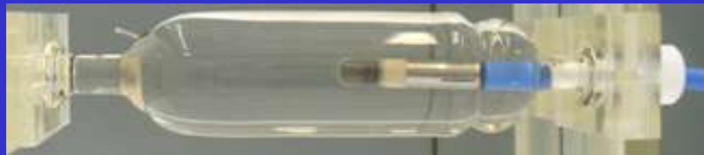
Vessel with an ion chamber
