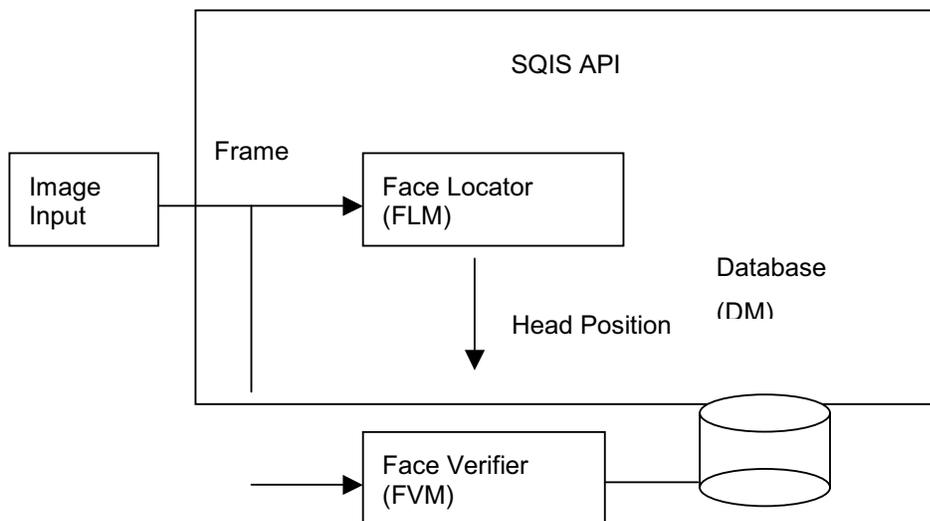
Figure 1: Block diagram for SQIS API
