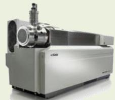
All sources coupled to an AB Sciex 4000 Qtrap Triple-Quadrupole MS
