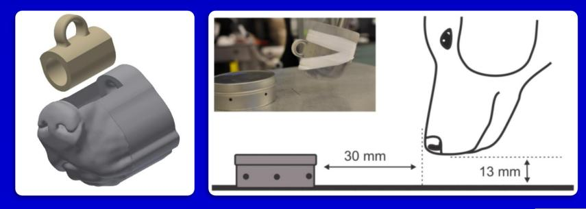
Experiments show a factor of 4 increase when the dog is sniffing vs. inhale only. During inhale, the dog nose acts as a potential flow inlet (with minimal aerodynamic reach). Exhaling air jets act to augment this limited reach via fluid entrainment.
