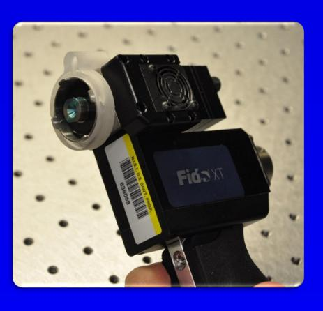
Designed and printed "nostrils" for COTS vapor detectors
