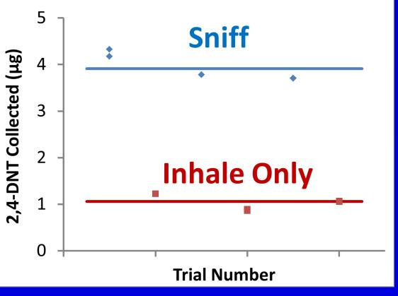
Artificial dog nose is more cooperative than a real dog in a schlieren system Jet-assisted sniffing (active) is used by the dog to augment potential flow inhale, thus increasing the aerodynamic reach for vapor a particle sampling
