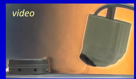
The dog is an *active* aerodynamic sampling system, using turbulent air jets to entrain fluid from ahead of itself.
