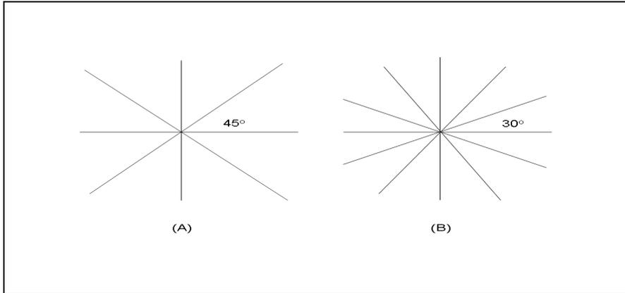
There are two possibilities. The test directions are four ways as shown in Figure (A) or six ways as shown in Figure (B).
