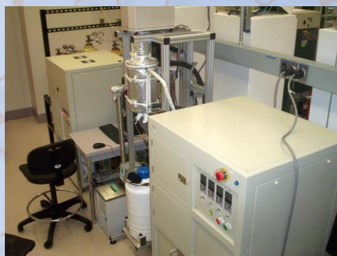
Multicomponent Gas Measurements. Instrument for binary gas mixtures (bottom right) and manometric instrument with gas chromatography for multicomponent gas measurements (upper left).
