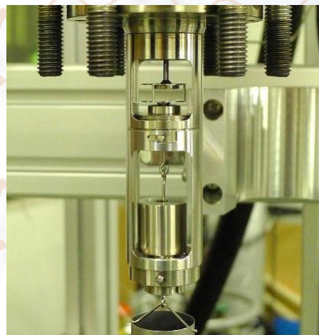
Binary Gas Adsorption Measurements. A magnetic suspension balance monitors mass uptake simultaneously with changes to the total pressure.
