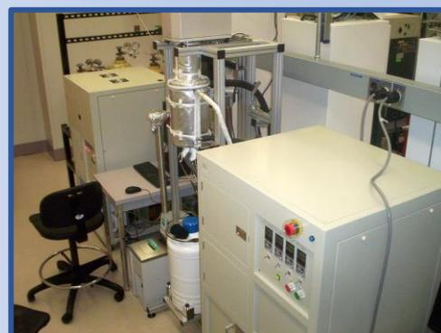
Multicomponent Gas Measurements. Instrument for binary gas mixtures (bottom right) and manometric instrument with gas chromatography for multicomponent gas measurements (upper left).
