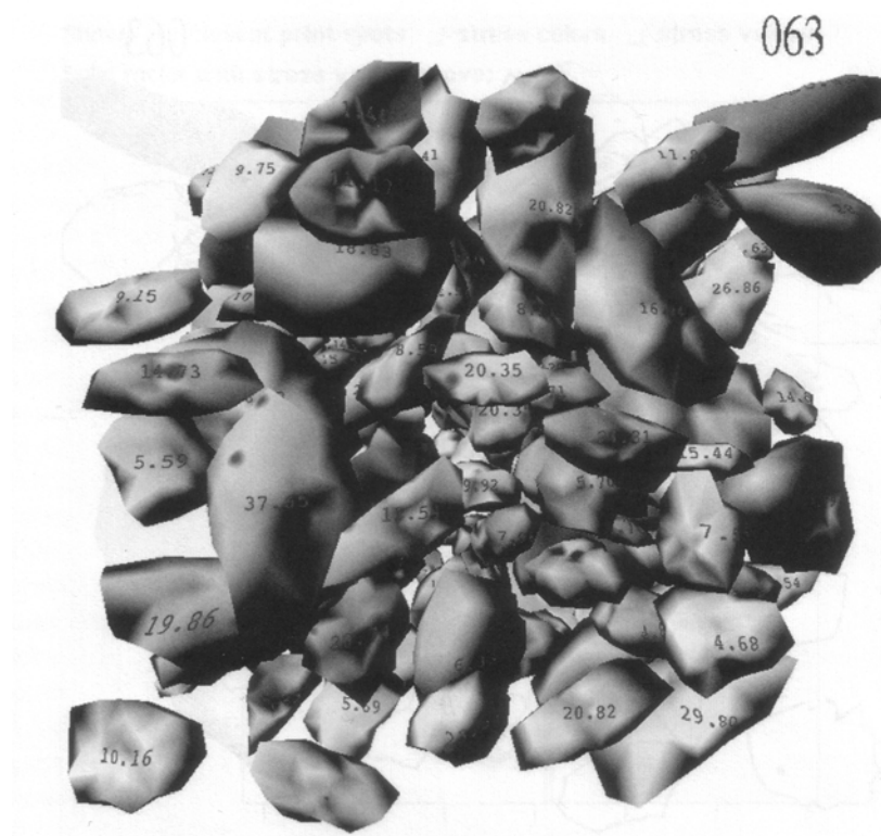
Fig. 13.3 Frame 63 in a simulation of the flow of rocks in a suspension. The per-rock stress is shown with a gray-yellow color scale, and also with a numeric value printed on the face for each rock (See Color Plates)
