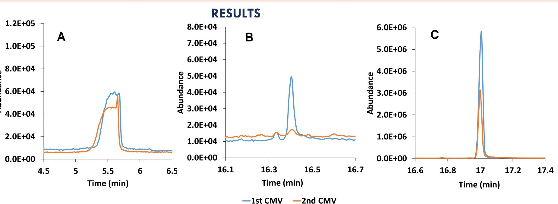
Figure 3. Chromatograms of overlapping responses of two CMV's in series following a 10 minute collection of generated vapors at a 500 mL/min flow. A) 2,5-dimethylfuran (RT = 5.181 min), B) tetradecane (RT = 16.405 min), C)  $\beta$  – caryophyllene (RT = 17.032 min).
