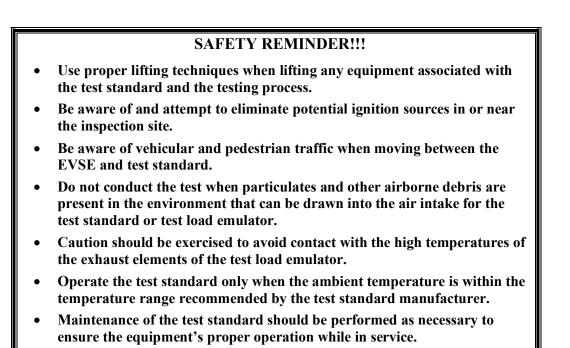
• There should be a clear perimeter and no site fixtures, other equipment, or landscaping that obstruct access to the test standard and the EV when used as the test load.
