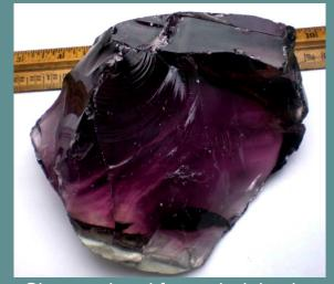
Glass produced from a high level radioactive waste simulant http://www.geologyin.com/2016/11/can-radioactive-waste-be-immobilized-in.html
