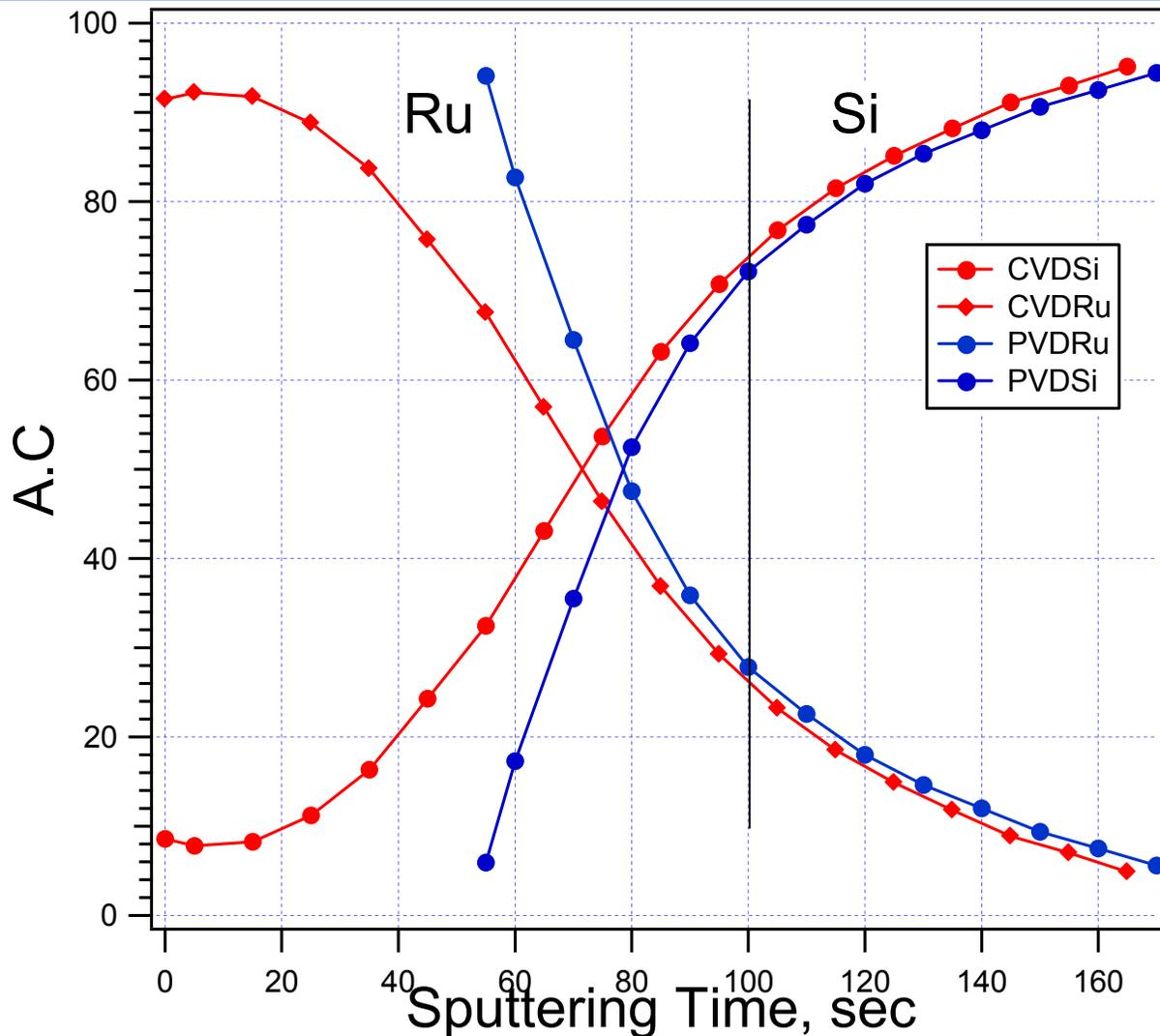
If we assume after the line is the interface, then the thickness of CVD film is 7.8 nm, calculated from from the sputtering time
