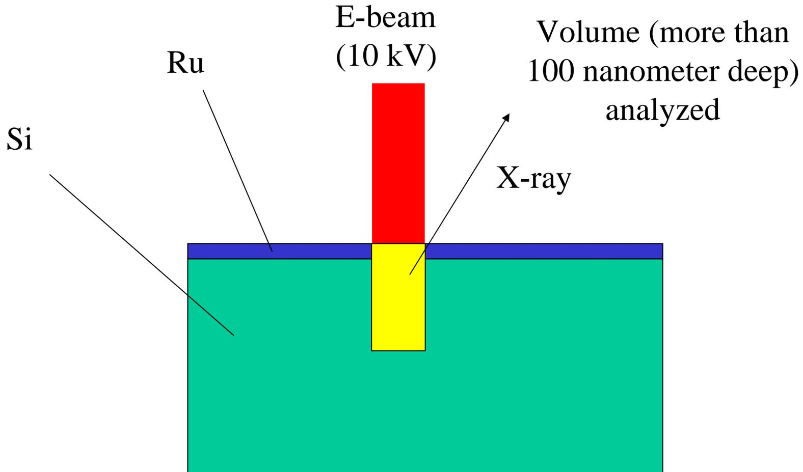
The detection depth of EDS is much larger than XPS, so it is not sensitive to the surface morphology
