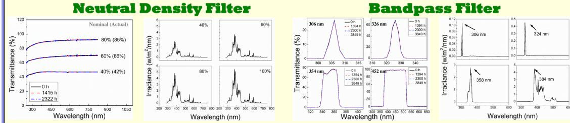
Both neutral density filters and bandpass filters are stable during UV exposure at 85°C/Dry on the SPHERE.
