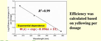
Efficiency was calculated based on yellowing per dosage
