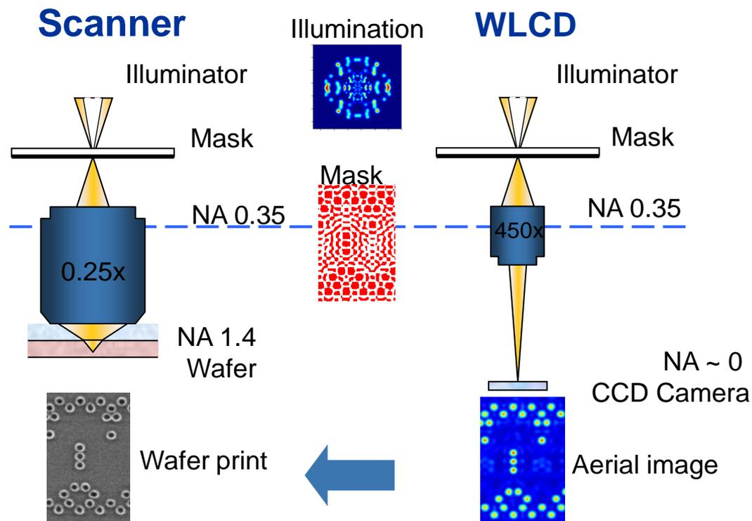
Equivalent image formation for Scanner and WLCD
