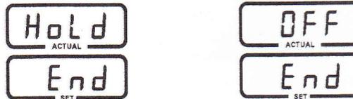
9. If the final temperature is to be held indefinitely at the end of the ramp and soak program, press **MODE** when "HoLd" is displayed on the Actual Display. If heater power is to be turned off at the end of the program, press **MODE** when Actual Display indicates "OFF." Proceed to step 20.
