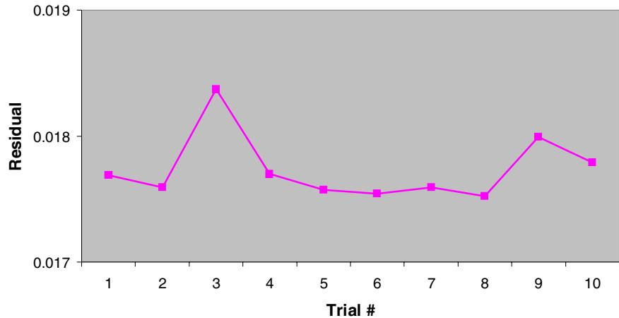
10 repeated trials, measuring 6 thicknesses and SiON dispersion for a DUVSE recipe for a Si-rich SiON/oxide/Si-rich nitride/oxide/Si-rich nitride/CuO/Cu stack
