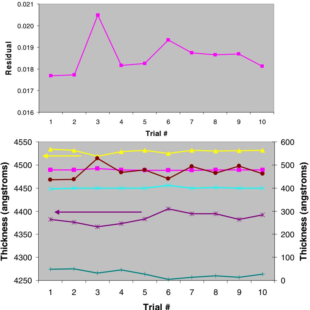
10 repeated trials, measuring 6 thicknesses and NIT1 dispersion for a DUVSE recipe for a Si-rich SiON/oxide/Si-rich nitride/oxide/Si-rich nitride/CuO/Cu stack
