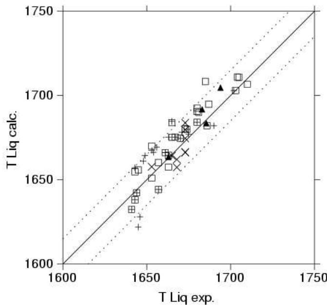
Comparison of the liquidus temperature calculated with the measured ones in the  $\gamma$  or  $\gamma'$  fields (the points where another phase appears during the calculation have not been considered).
