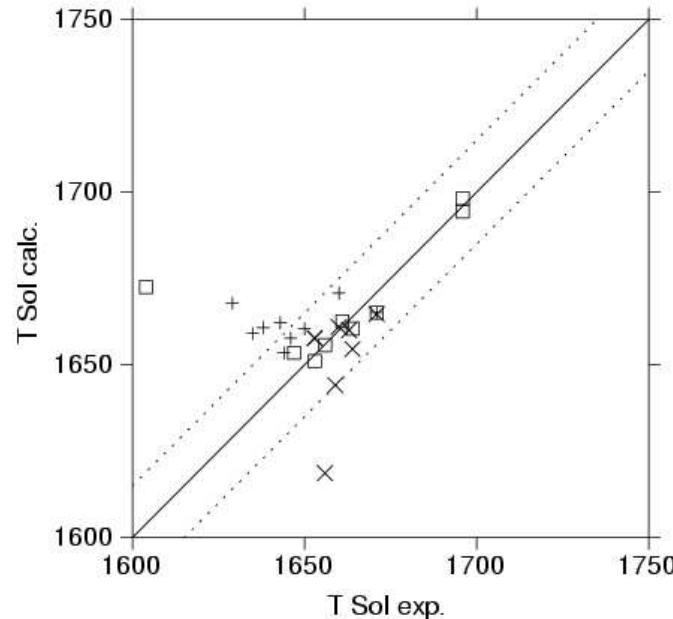
Comparison of the solidus temperatures calculated with the measured ones in the  $\gamma$  ou  $\gamma'$  field (the points where another phase appears during the calculation have not been considered).
