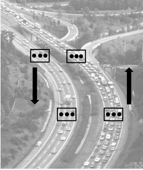
**Figure 6:** Traffic zones are an aggregation of traffic lanes. The dots are traffic lane detectors and the boxes are the traffic zones. In this figure, there are 12 traffic lane detectors: 4 traffic zones with 3 detectors in each zone. There is one traffic zone detector per road segment in each direction. In the data, there are different numbers of lane detectors in each traffic zone. This photo was obtained from National Archives [6].
