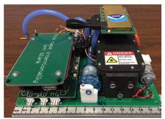
NOAA CSL's Portable Optical Particle Spectrometer (POPS) uses an on-board laser to measure tiny suspended particles that influence stratospheric chemistry and reflect incoming sunlight. The miniaturized instrument, designed by CSL researchers in Boulder, Colorado, weighs 1.3 pounds and is about the size of a lunch box. Credit: NOAA
