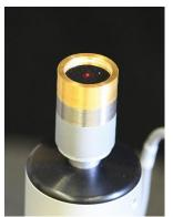
Close-up of a microphone, with the laser spot hitting the center of its diaphragm. Credit: NIST
