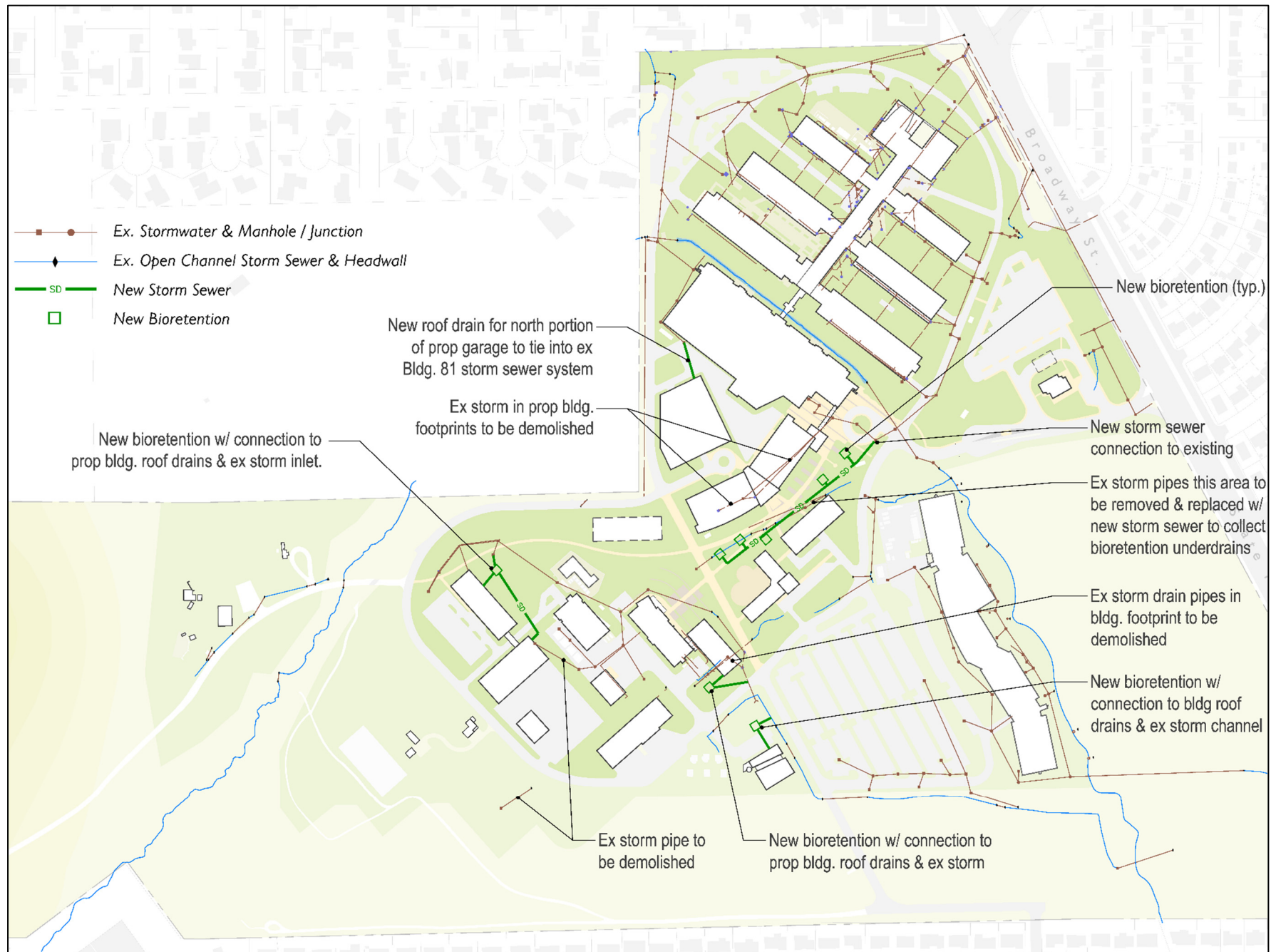
Figure 4-4. Proposed Stormwater Conveyance Network under the Master Plan
