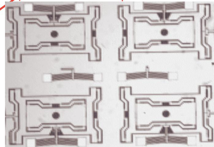
Array of 2D Si MEMS prototypes (vs. #2)
