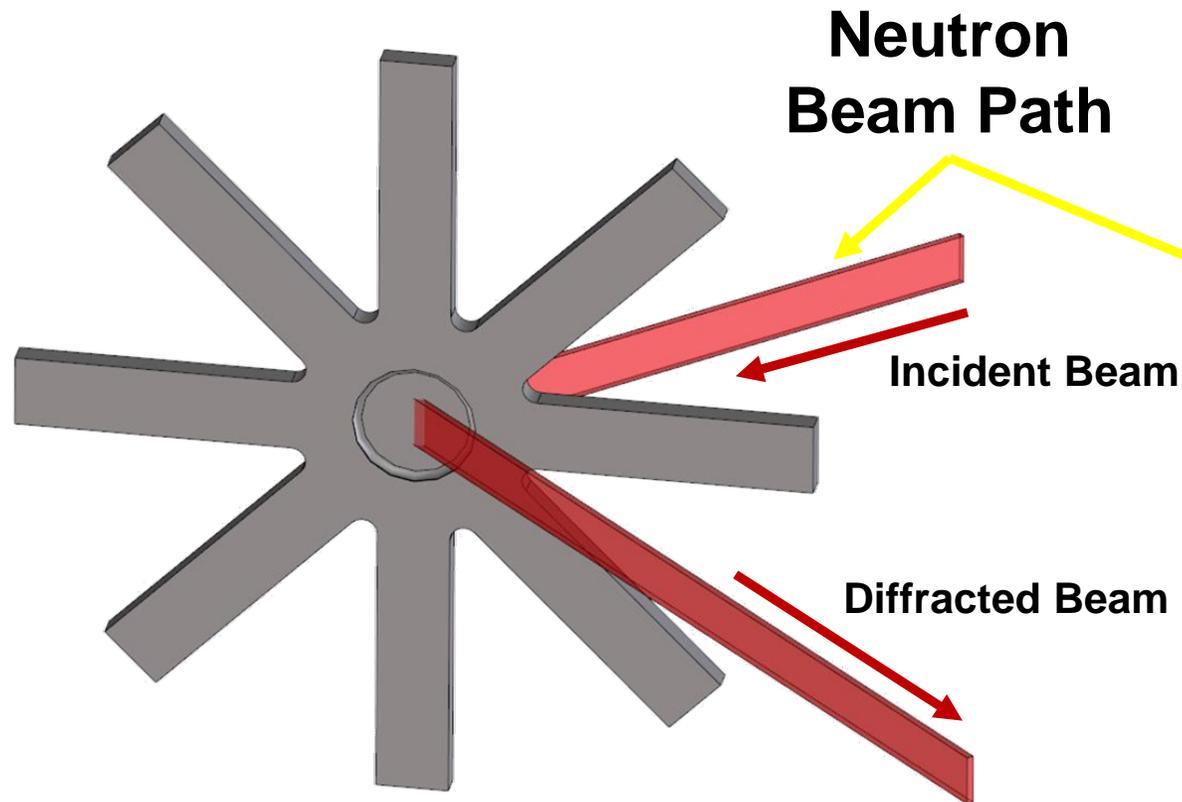
Figure 10: CAD model of Octo-Strain Test Specimen
