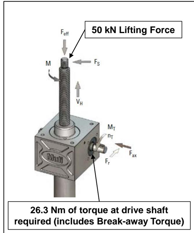
Figure 15: Free-body diagram of forces acting on screw-jack [4]
