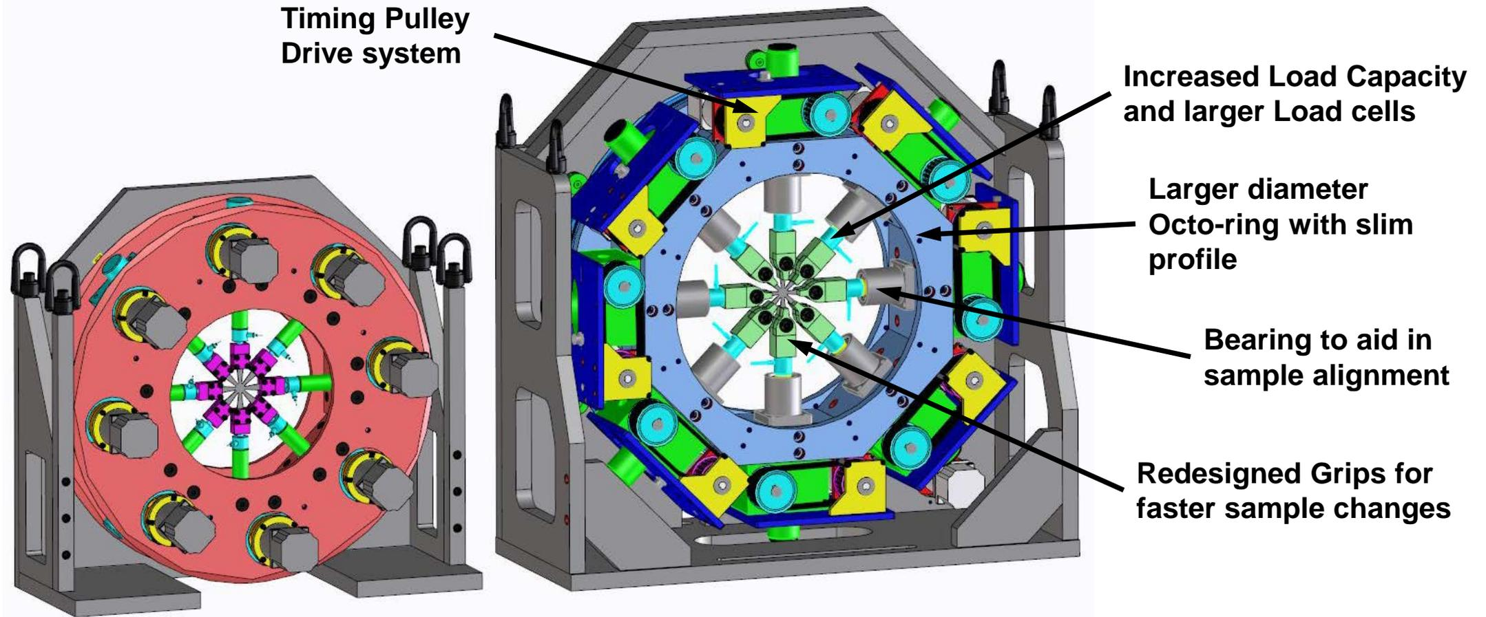
Figure 23: CAD model of 50 kN redesign compared to existing 10 kN design
