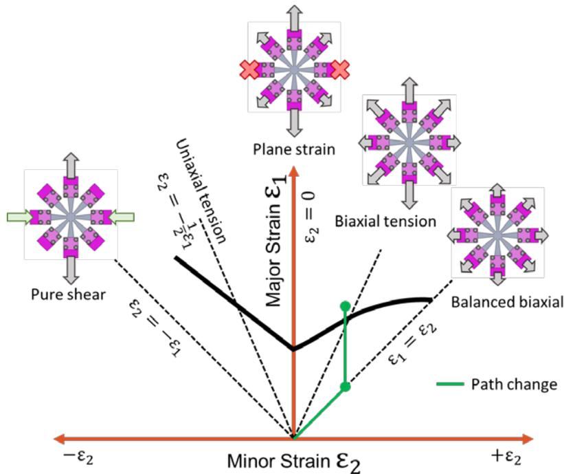
Figure 2: Various Strain Paths for Octo-Strain Device
