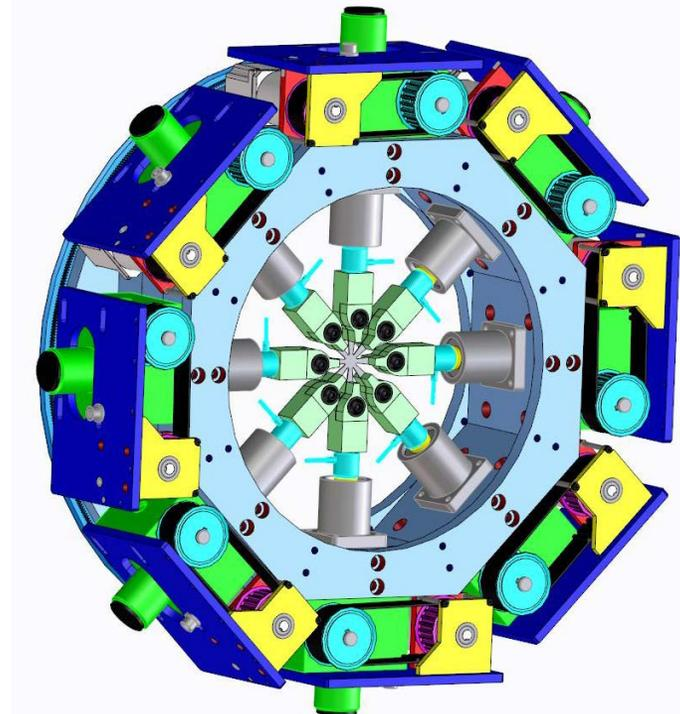
Figure 19: Assembled Octo-Ring without Test Stand
