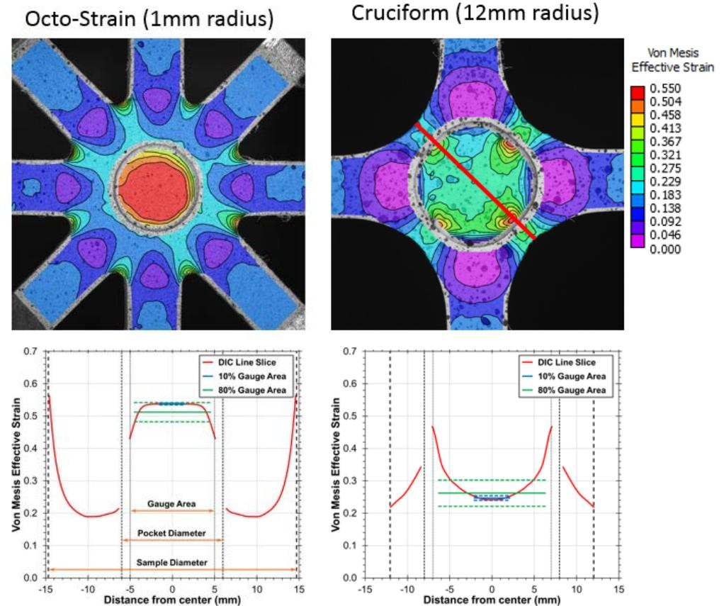
**Figure 12: Strain Path of Octo-strain test specimen and cruciform**
