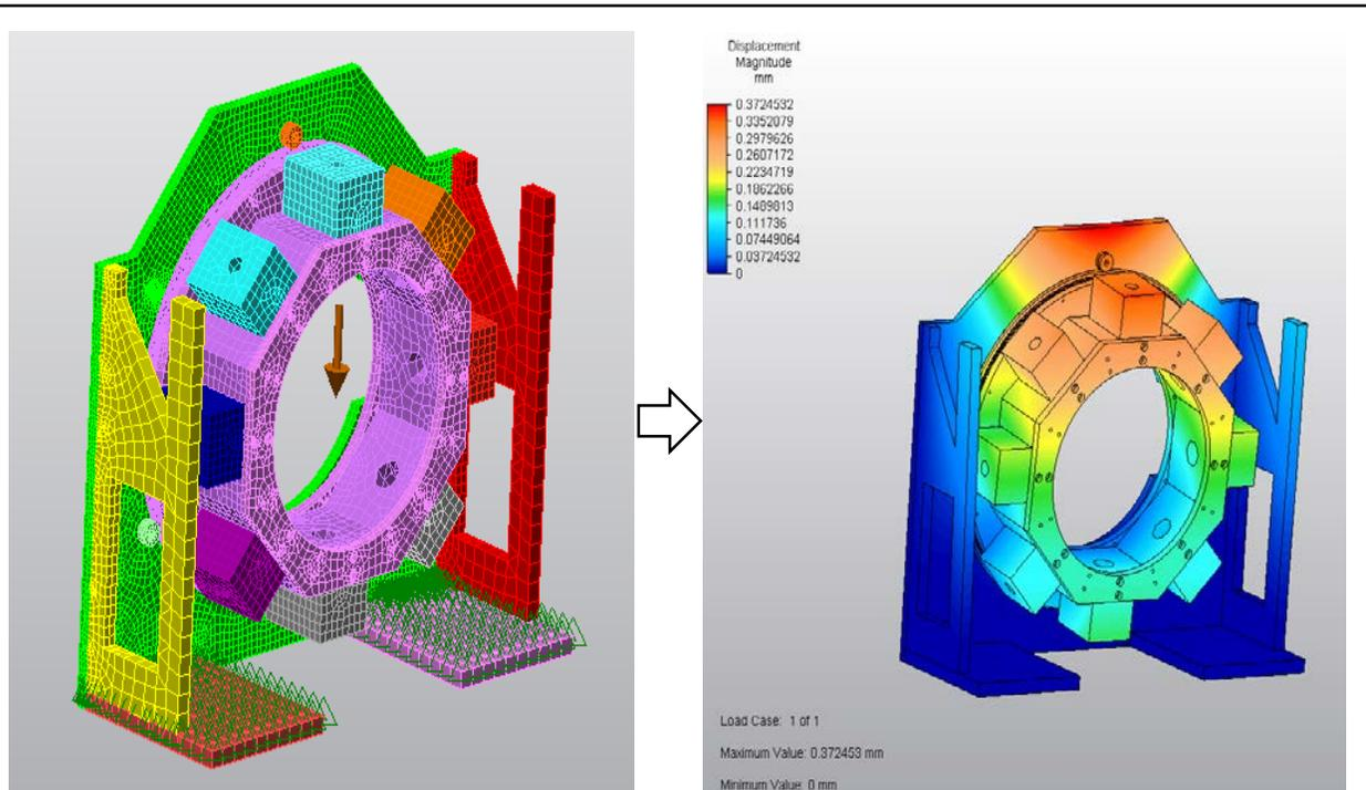
Figure 18: FEA Result of Max. Deflection due to gravity (0.37mm)
