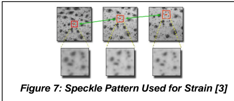
Figure 7: Speckle Pattern Used for Strain [3]
