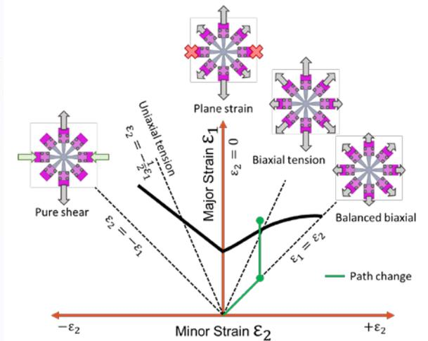
Figure 5: Strain Space for Octo-Strain [2]
