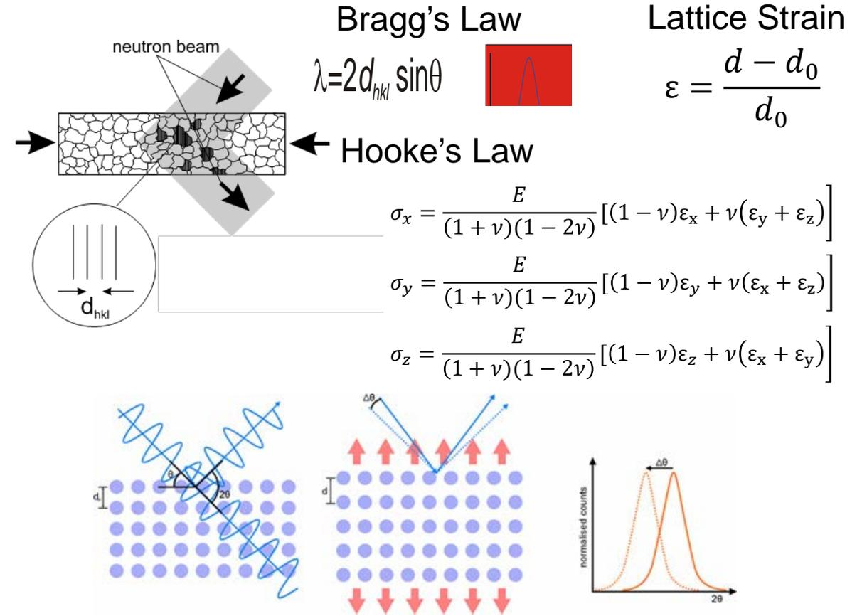
Figure 9: Finding Stress using Neutron Diffraction
