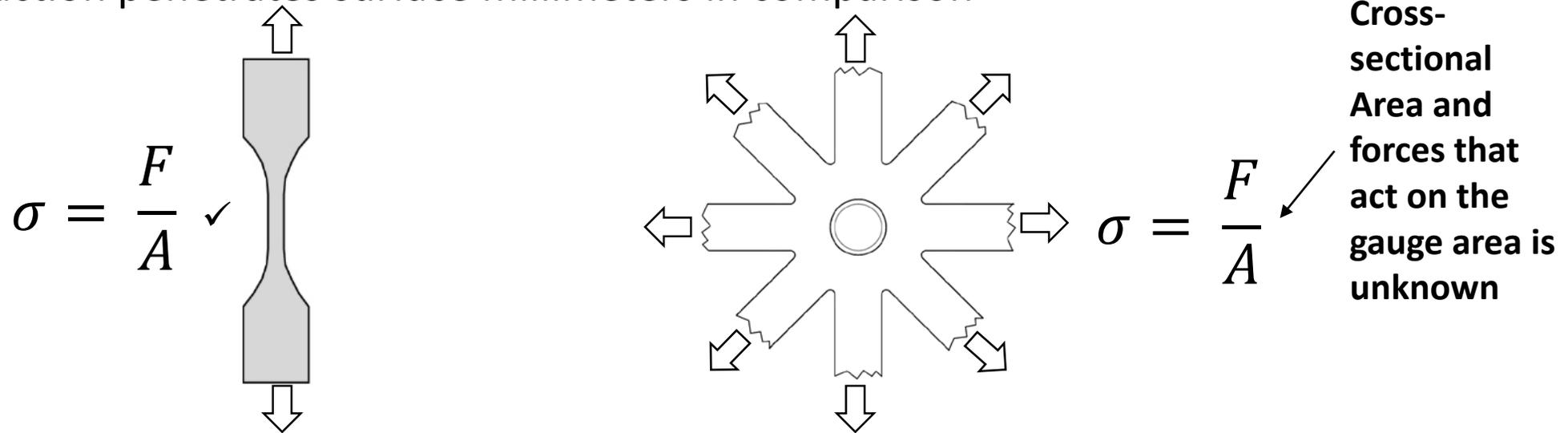
Figure 6: Comparing traditional tensile test specimen to Octo-Strain test specimen
