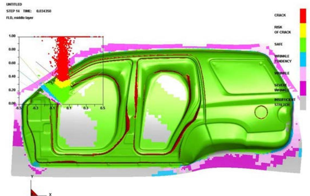
Figure 3: Strain Paths when Forming Automotive Parts
