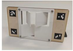
We use a set of easily-produced 3D printed and lasercut fixtures to measure depth quality. Simple geometries that approximate real-world objects in manipulation environments assess depth quality better than manufacturer metrics, which are often measured against flat walls. Known fiducial locations make the fixtures easy to align during processing.
