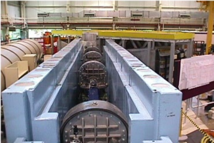
Chopper housings, looking toward the DCS instrument (under construction)
