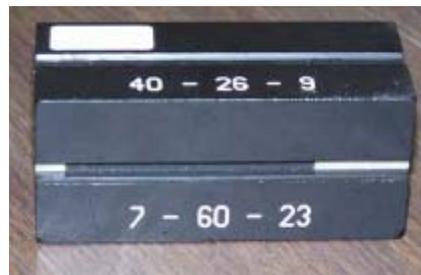
**Test block (reference standard) used for calibration and testing of a Fat-O-Meater**
