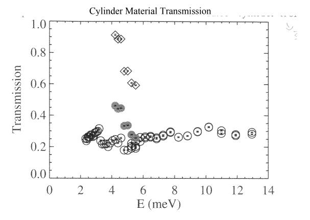
Circles: Transmission through the  $ZrO_2$ Squares: Transmission through the  $Al_2O_3$ Open: Measured with PG(002) filter, 20' collimation Closed: Measured with PG(002), 80' collimation
